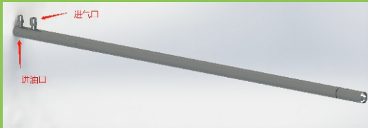
自制内混式油枪 Self-made internal mixing oil lance
